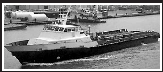
Miss Jenney 65' x 22' 800 HP, Twin GM 12v71's MG 514 (6:1) Flk Rudders; Elect. Winches; RCP.
