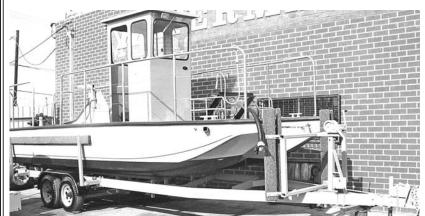
Manufactured by Willard in 1997. Powered by Volvo diesel, Model AD31L130 with a DPDI dual prop outdrive.
