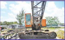
GM6V71 Diesel, Env. Cab, Air Controls, Power Load Lowering, Tracks 15'4" L x 13'2" W w/30" Pads, 100' Angle Boom, Hook Block, Rear Folding Gantry, External Removable Counterweight 18.000#. Full Revolving Fairlead. Machine Weight -91,140#. Completely Operational. Price: Located In West Palm Beach, FL
