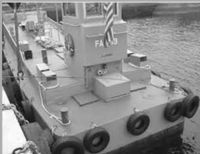
1993 15 Meter Work Boat — 15MWB9201 Builder: Gulf Copper Hull: Steel Twin Cummins Inboard Engines
