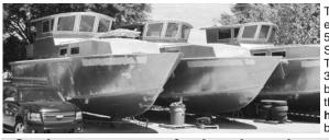
These units are built to the highest standards. Hull: Schedule 5086 5/16 plate. Superstructure: Schedule 6061 & 6063 plate. They were part of an order for 30 vessels but a change in the buyer's circumstances caused the cancellation. \$240,000 per hull as is, or completed to buyer's finished specs.
