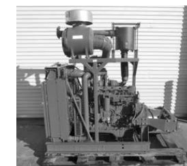
QSB 6.7 Cummins Power Unit 260HP, SN# 46941797, CPL 8611 260HP @2200RPM, MFG 2008 $20,000
