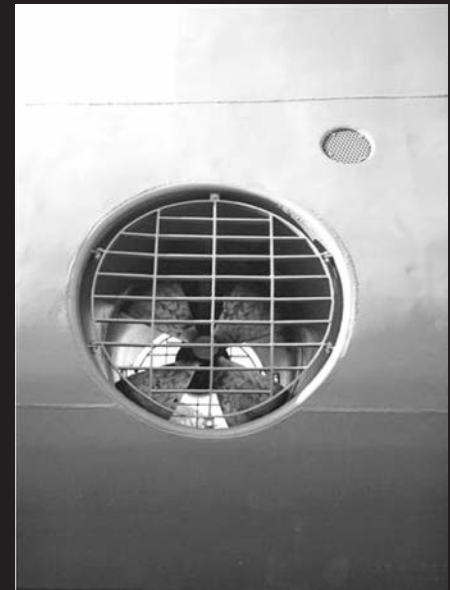
HYDRAULIC DRIVEN BOW AND STERN THRUSTERS FROM 50 HP TO 650 HP
