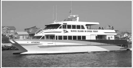
100' x 30', 250 passenger ferry certified for limited coastwise routes. This vessel has a service speed of 30 knots and has active ride control. Powered by (4) 3412E Caterpillar mains and Hamilton Water Jets. Passenger comforts include A/C, heat and Satellite TV.
