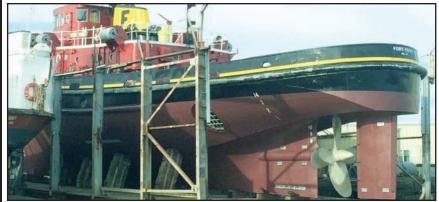
Ex Navy YTB 102' x 29' x 14' - 2,000 H.P. Single Screw Tug with 800 H.P. Stern Thruster. Main Engine: Fairbanks Morse 10-38D 8 1/8. SMI 52" tunnel thruster driven by Detroit 12V-92. (2) 6-71 75 KW gen sets. 3,000gpm firefighting system. Last dry dock July 2015.
