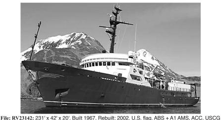
Sub "U", "I", COI, SOLAS. Dwt: 1,800T. FO: 105,000g. FW: 16,000g. 15T & 5T cranes. 10T A-frame. M/Es: 2 x EMD total 2,400HP o'hauled 2002. Speed 12.5-14kn. Range 10,925nmi / 45 days. Bow thruster. Gensets: 2- 300kW; 1-75kW. Quarters for 48 in 7 single & 20 double cabins + berths for up to 11 crew. AirCon. Hospital, lounges, wet lab, conference & data process rooms. Mess seats 34. 2 watermakers. Commercial grade incinerator & laundry room. Anti-roll system.
