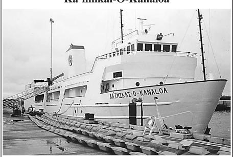
File: RV22338: 223' x 38' beam x 16' depth / 13.5' draft. Built 1979 by Mangone Shipbldg. as Seismic Vessel. Lengthened / modified 1991 – 93 for oceanographic research / manned submersible support. U.S. flag. GRT: 259. ABS +A1, AMS current thru 30 Aug. 2018. FO: 91,000g.
