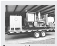
Seven rental generator units on trailers: 250kw, 225kw, 99kw, 65kw, 40kw, and two 30kw units
