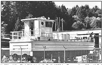
**File:** UB05016 50' x 14' x 7'. 1.5' light draft. Built 1989 by Oregon Iron Wks. U.S. flag. Lt. Disp: 30st. 20' x 11' x 5.75' well deck. FO: 560g. 2 x GM 6-71N total 348BHP. TD 1.48:1 gears. New recessed 24" x 14" props on 2" stainless shafts. New controls. 24vDC electrical. Radar. 1 berth. Heavy push knees. New aluminum pilothouse. Last drydocked June 2018. New 3/16"
