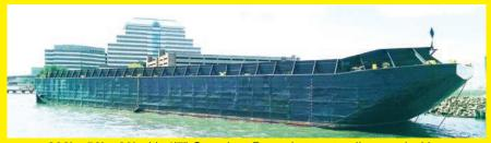
266' x 56' x 20' with 4'7" Coaming. Barge is structurally sound with a double bottom and is ready for work! Cargo capacity is approximately 5,000 short tons, non loadline. Fresh off of long term charter and just out of the shipyard. All exterior coatings and zincs have been replaced.
