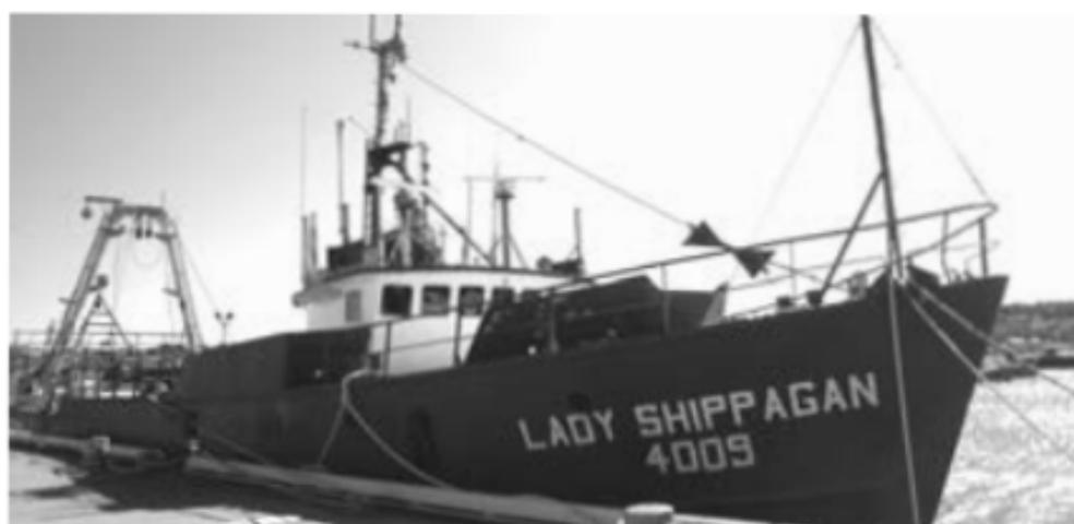
126' Steel Stern Factory Trawler with Cat D399 built in 1975. Nice for yacht or freight project, hull perfect, ice class. - **\$175,000 USD**
