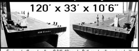
Equipped w/2 spud wells, w/2 24"x40' spuds. Both spud wells equipped with Nabrico DF-1-65-11L winches w/60 ton capacity. International Load Line Certificate. All void tanks and internal framing recently reworked to support heavy deck loads. Tonnage plates installed in 4 voids for ABS and USCG certification.
