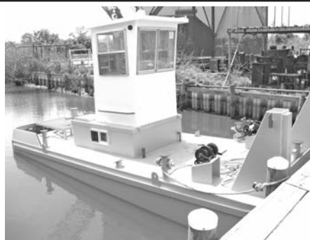
MODEL 2510 25'9" x 10'0" x 4'0" 200 H.P. Single Engine
