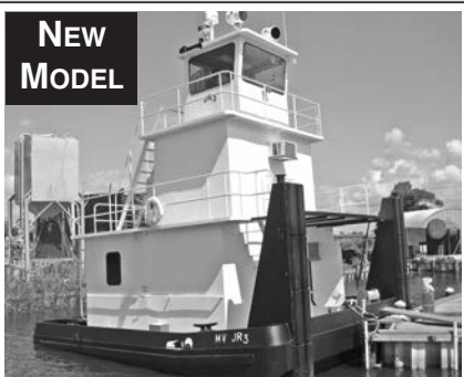
NEW MODEL MODEL 2523 with Quarters 25'9" x 23'0" x 6'8" 975 H.P. Triple Engine
