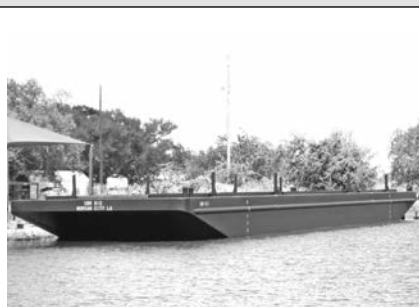
DECK BARGES 120'0" x 30' 0" x 7'0" Double or Single Rake
