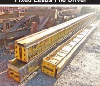
Three Sections, Head Section 30 Ft., Spoter Section 30 Ft., Mid Section 20 Ft., Total 80 Ft.
