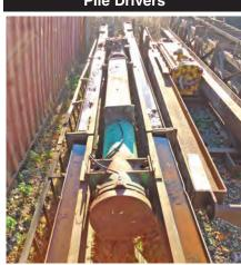
Diesel Hammer With 40 Ft. Of Hanging Leads, Spare Parts (Injector), Started And Ran When Last Used.
