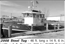
width x 5 ft. Draught, 350 hp 8V7IT Detroit Diesel w/ 5114 3:1 Twin Disc gear, 3 in. shaft with 38 in. x 32 ft. 4 blade Nibral propeller. It has a 7.5 kw Onan generator and full electronics. Pilot house is removable for transporting. Asking \$450,000.00 Canadian Dollars Located in Ontario, Canada Contact Numbers Are:
