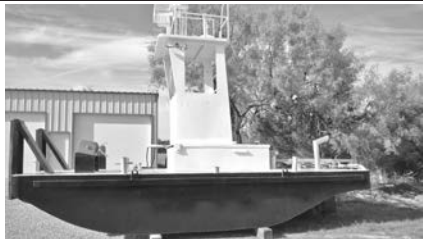
20' Push Boat, 471 Detroit, ZF 1.5 Gear, Keel Cooled, Flanking Rudders, 80 Gal. Fuel, 15' 6" Eye Level.
