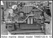
liter 400 horsepower @ 1800 RPM, with Twin Disc 5111 marine transmission 4:1 reduction. New head, fuel injection pump, injectors and turbo. Engine and gear like new. Run exclusively in fresh water on tour boat. Includes instrument panel and all wiring.
