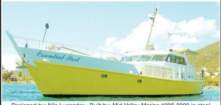
Designed by: Nils Lucander • Built by: Mid Valley Marine 1999-2000 in steel LOA 65ft - DISP. 138,000lbs - DEPTH 6ft - BEAM 22ft - Fuel 3,200 Gal. Water 480 Gal. - Twin Isuzu 6cyl. w/Hurth 4.5:1 w/PTO to Hydraulics, 40" wheels Norpro 20KW - Wind Gen. - Large Solar array - Boston Whaler w/15 Very substantial ground tackle - Hydraulic winches - Asking \$350,000
