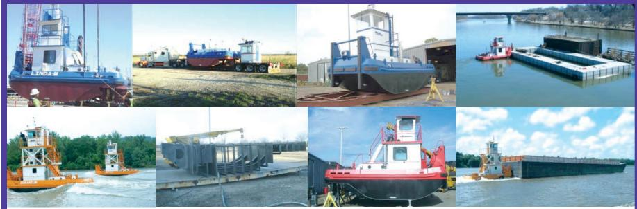
True 18" Marine Framing, Multiple Bulkheads and Shipped Complete and Ready For Action With All Required Equipment Plus Navigation Lights, Horn, Radio & Wiper.
