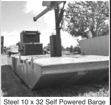
Steel 10 x 32 Self Powered Barge With Cummins.
