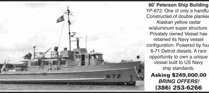
YP-672. One of only a handful. Constructed of double planked Alaskan vellow cedar w/aluminum super structure. Privately owned Vessel has retained its Navy vessel configuration. Powered by four 6-71 Detroit diesels. A rare opportunity to own a unique
