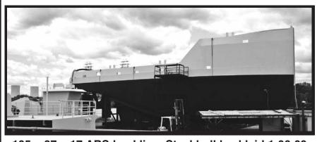
105 x 37 x 17 ABS load line. Steel hull keel laid 1-06-09 designed for 3516 all steel work for houses/hull complete. Shafts included.
