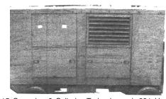
MB-15 Cummins 6 Cylinder Turbocharged, 891 Hours, 24 V Starter, Model NTC-6, Trailer Mounted, 8,000 Lbs.
