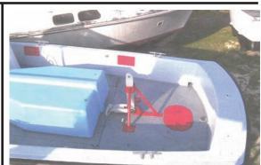
37' x 13' - Standard Stern View Showing "HD" Towing Bitt That Is Secured Under The Deck To The Main Horizontal Beams.
