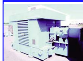
ASEA Synchronous 10,200 H.P. Motor
