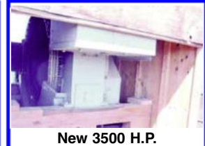
New 3500 H.P. G.E. Synchronous Motor Model #131151 - RPM - 276.9
