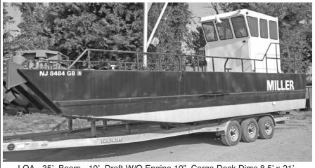
LOA - 35', Beam - 10', Draft W/O Engine 10", Cargo Deck Dims 8.5' x 21'. Cargo Door Dims 8.5' x 3', Raised Wheelhouse Dims 6' x 5.5', VHF Radio, Spotlights, Work Lights, Manual Davit, Drive On Galvanized Tri-Axle Trailer, Towing Height On Trailer 13' 3, And Honda 225 Outboard.
