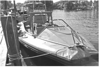
LOA - 32', Beam - 9'6", Draft 18", Operational Draft 24", Engine: Cummins 6BT 300 HP,
