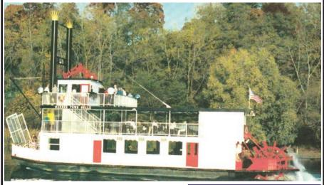
Built to ABS standards. On land for USCG 5 year inspection Feb.-May 2014. Working smoke stacks no diesel smell. 3ft draft - no running gear below flat bottom. Twin Cummins 6 BTA 5.9 diesels. Twin 65KW Nothern Lights gen-sets.
