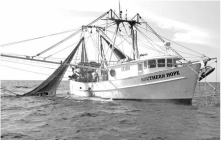
3408 DIT 500 HP, Twin Disc 4.5 to 1 Gear With Kort Nozzle 45 KW Gen Set, Blast Freezer Brine Tank, Garcia Winch Auto Pilot, A/C Draft 9.4" Fuel 5500 Gals., Water 1500 Gals. Rigs 4x40' - 8' Doors
