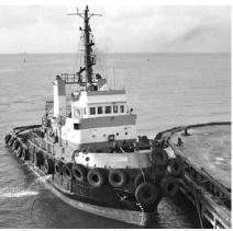
Blt. 1976, Japan, Niigata 2500 BHP, Twin Screw, Single Drum Winch 600 Mtrs. x 48 MM, Dim. 34.02 x 9.20 x 4.24 Mtrs., Inspectable Caribs.
