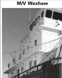
70' x 24' • 1,350 hp • Built 1973 Cummins KTA-38 Engines
