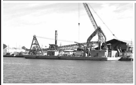
Aggregate Unloader Barge "Big 903" 145' x 42' x 8' - Capable of unloading 700 tons up to 4" diameter rock per hour, Caterpillar 375L Material Handlers #IJM00532 w/ 5 yd bucket, 125' of conveyor, can load directly onto trucks, hoppers, and shore, JCB 406B wheel loader #DEC 1S127/ SN: 1300961.
