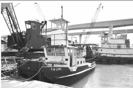
**R.B. Long - 400 HP Day Boat -** Hull Number 26504 • Milwaukee, MI • 37.2' x 12.3' x 5.0' Towing Vessel. Total refurbish 2013 including new running gear, shaft, props, bearings and hydraulic system. V8-71 GM with low hour and 3-1 Twin Disc 509 Gear • 43' x 36'.
