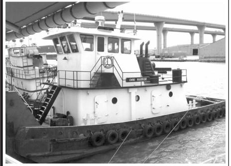
**Omni Warrior** - 1200 HP Push Boat • Hull No 614866. Registry: New Orleans 51.5' x 22.0' x 8.6' • Net Tonnage: 62 N.R.T • Towing Vessel • Eye Level: 20' • Fuel: 9500 Gal.. Water 6000 Gal.
