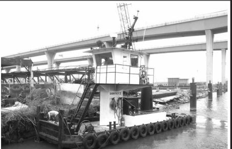
**Danny Boy II** - 400 HP Day Boat • Hull No 519558, Registry: New Orleans • 36.5' x 14' x 4.70' • Net Tonnage 63 N.R.T. • Towing Vessel
