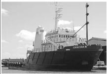
880 Gross Tons, 170' x 40.5' with a breadth of 18.37', 236,000 gallon fuel capacity, accommodations for 30, 7,374 bhp horsepower. Class status laid up.
