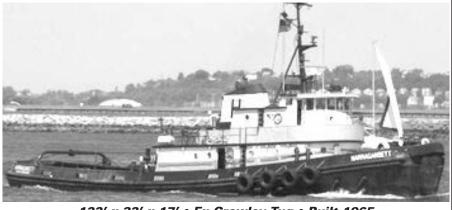
122' x 32' x 17' • Ex Crowley Tug • Built 1965 M.E. Turbo EMD 16-645 • Falk Gear 4.5 To 1 Prop. 122 x 98 - 5 Blade • Cat Generator Sets Fuel Cap. 60,000 • Water 18,000 • Sleeps 8 • 2 Heads Almond Johnson Winch 2000' Of 2" Wire • Full Electronics Current A.BS. Loadline Good For 2 More Years Ocean Service Just Off Contract • Great Sea Boat
