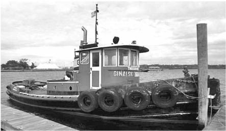
Designed and built by Gladding-Hearn in Somerset, MA. She is a single screw steel hull harbor tug powered by a naturally aspirated 400 HP Detroit 12V71 diesel engine with 2,504 hours on the meter. Year Built: 1960, Vessel Name: Theodore, USCG Doc. No.: 281193, Ship Builder: Gladding-Hearn, Length (ft.): 40.5, Hull Depth (ft.): 5.8, Hull Breadth (ft.): 13.2 Gross Tonnage: 17, Net Tonnage: 11
