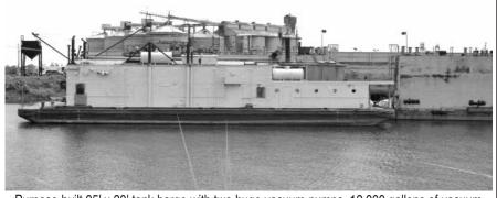
Purpose-built 95' x 30' tank barge with two huge vacuum pumps, 12,000 gallons of vacuum tanks, able to provide tremendous volume of vacuum for skimmer, cleaning operations.
