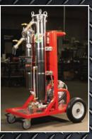
Mobile Systems Remove: Sludge, Water, Bacteria Fungus Contamination From Diesel Fuels.
