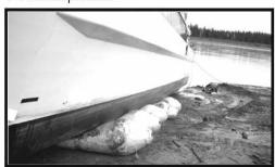
3' x 13' Hypalon air bags for lifting & rolling marine vessels. 10 ' of lifting surface. Air pump available with manifold to inflate multiple bags at once.
