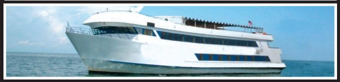
**154' x 40' x 7'** - Licensed to 415 Passengers, Can be Raised to 600 Plus Pax, 20 miles USCG, 2 Walkins - Coolers/ Freezers, 20,000 Gal. Fuel Capacity. Main Engine Wings 3412 Center 3508 All Keel Cooled - Cats • (3) 3304 90kw Cat Generators, Bulbus Bow Bow Thruster. Hydraulically Operated Mast Allows Airdraft Down to 30'. (2) Extra Large Bilge Keels For Super Stability. All Engines Are Running and Ready For Sea Trials. This Vessel is Ready to go to Work.
